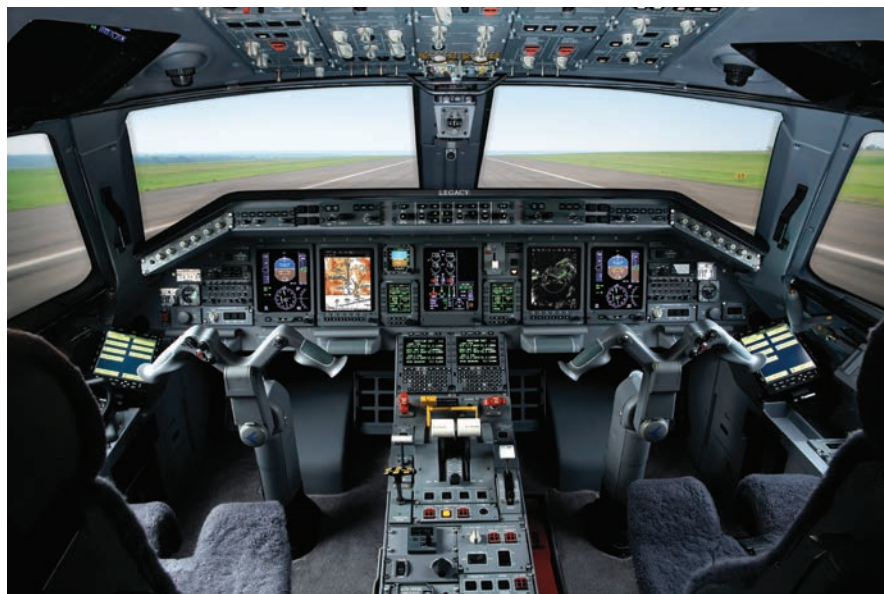
Honeywell Primus Elite features five, 8-by-7-in. LCD screens. The layout has left- and right-side PFDs and MFDs, along with a central EICAS.
