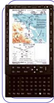
the EPOP (Embraer Portable Operational Package) notebook-based software with performance, weight and balance and electronic documentation (Publication Viewer) capability to fit the hardware class that is required for running on the EFBs.
