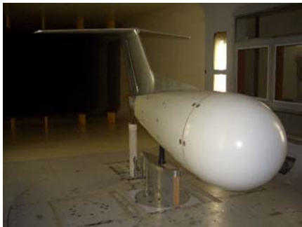
Phenom 100 in Wind Tunnel at Brazilian General Command for Aerospace Technology (CTA)
