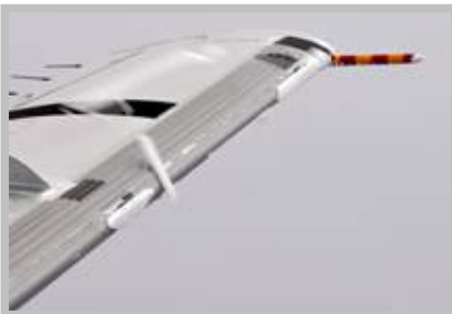
Icing test: the moment when the wing booth broke the ice.
