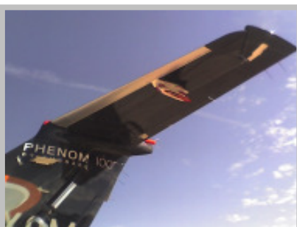
The Phenom 100 with flutter vanes installed
