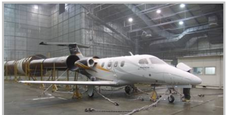
The fourth Phenom 100 performing cold soak test at Eglin Airspace Base
